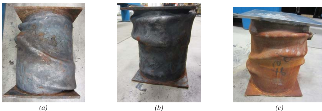
Fig. 4. Failed stub columns: (a) SC1; (b) SC2; (c) SC3.
